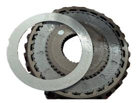
i. Remove the clutch pack, roller bearing: Make note of the shim location, remove and reinstall later. The actuator may fall out, or it may remain in the side cover. If it falls out set aside for reassembly.
