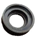
**Remove the center splined insert in the clutch pack:** To do that, first remove the thin circlip that retains the clutches. Then carefully remove the center splined insert. Reinstall the circlip
