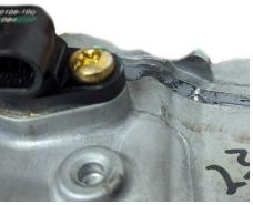
h. Remove the Passenger Side Differential Cover: This side is a bit harder to remove as it has silicone and not an o-ring. Unbolt the cover and use a dead blow to tap the cover off at the cast tabs. Then use large flat head screw drivers to pry the cover off.
