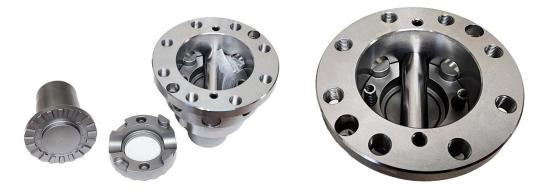
e. <u>Install the TORQ Locker Springs:</u> Lift off the upper axle gear and cam gear and install the 2 TORQ Locker springs into opposing cam gear, facing up. Place the upper cam gear on the springs so the springs go in the holes. Place the axle gear on the cam gear.
