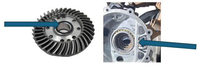
**a.** Make note of any shims found inside the housing: Remove the shims and keep them clean for reinstallation
