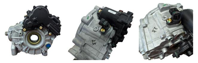
a. Remove the actuator: (4) T-30 bolts, three on the side, one on the top. Be mindful of the splines.
