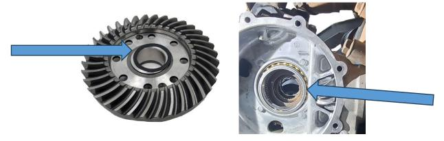
**a.** Make Note of any shims found inside the housing: Make sure each shim is reinstalled in the housing and on the locker case
