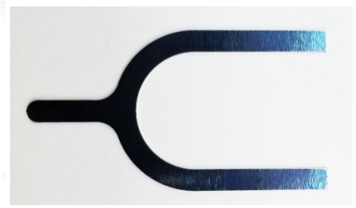
- u-shaped tool to remove circlip
