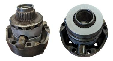
7.) Place the second Side Gear on the stack, then place the spacer on the Side Gear, then Bolt Case and Ring Gear back together Make sure to line up index marks.
