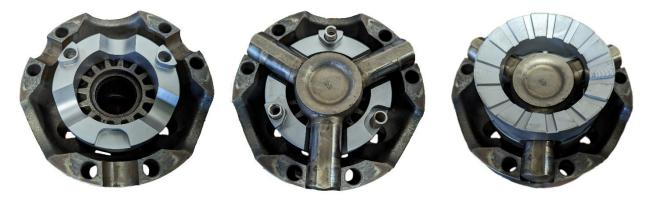
**6.) Drop-in the Cam Gear, Springs, Cross Pin, then second Cam Gear:** Use a little bit of grease to hold the springs in.
