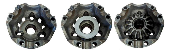
**5.) Drop-in the Spacer and Side Spider Gear:** Check the inside of the case for any remaining washers, remove if found.
