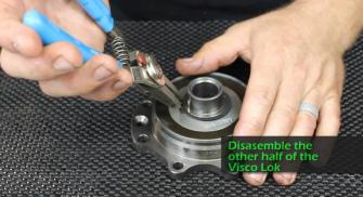
o. Open the other half of the Visco: You can push out the seal from the inside of the Visco case
