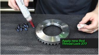
bb. Install The Ring Gear, Align the Index Marks: Torque Specs on ring Gear Bolts is 27 lbf-ft
