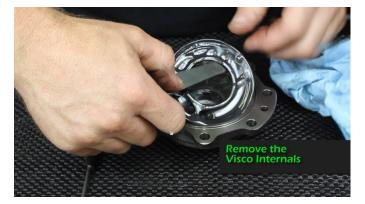
. Wipe out the Viscous Fluid completely
