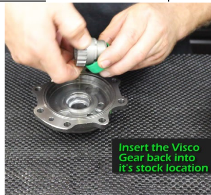
Use Gear Oil to lubricate the Visco Gear
