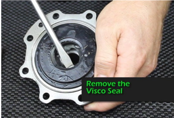
h. Remove the Visco Seal
