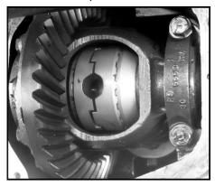
7.) Install the Two Springs: rotate the locker assembly and install the two springs into the Spring Pockets.
