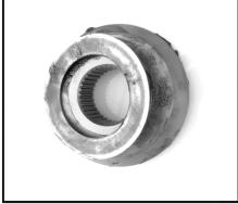
4.) Install Axle 2 Gears: with Thrust Washers on the backs of the axle gears, driver and passenger side
