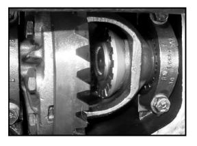
5.) <u>Install First Cam Gear:</u> on Ring Gear side of the case, push it into the grease on the teeth to hold it in position. Notice that next to one of the curved recesses there are pockets that must be facing outward.
