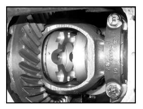
6.) <u>Install Second Cam Gear:</u> positioning it so that its projections will slip into the opposing pockets. Slide it in past the left connector until they are flush with each other. Push the right rotor into the grease to hold it in position.
