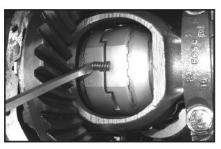
**NOTE:** The springs are Heavy Duty. Try using a flat screwdriver to pry the springs into the pockets. An alternative method is to compress the spring with pliers and insert it about half way into both cam gears, release the pliers, and then tap it into place with a screwdriver handle.
