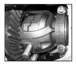
9.) Check the Center Gap Measurement: Use your caliper or feeler gauges to measure the gap between the two cam gears with the locker teeth engaged. This is an installation check to see if the thrust washers were installed or to see if the differential case is within average machining tolerances or if it has become worn. If the gap is out of specifications, please contact Customer Support: <a href="Info@TorqMasters.com">Info@TorqMasters.com</a>
