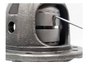
8.) Install the Pins and Springs: Pins go in the hole, springs go in the slot. The nub on pin retains bottom loop of spring. It's helpful if you use the nub on the pin to hold the spring in place, then use a small screw driver to compress the spring and pop it into the slot. It's critical to install the pins and springs in the correct orientation. Failure to install in the correct orientation could lead to severe damage in the differential.
