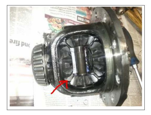
This is the spider gears we will be removing
