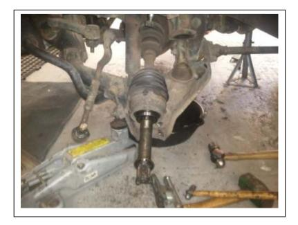
Finally the knuckle removed now you need to give a strong pull to release the drive shaft be careful if your vehicle is on a jack, do not let the splines of the shafts damage the seals
