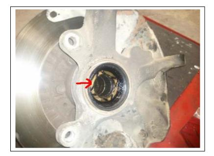
Note this washer will fall out when you separate the shaft and knuckle the pattern side faces towards the shaft
