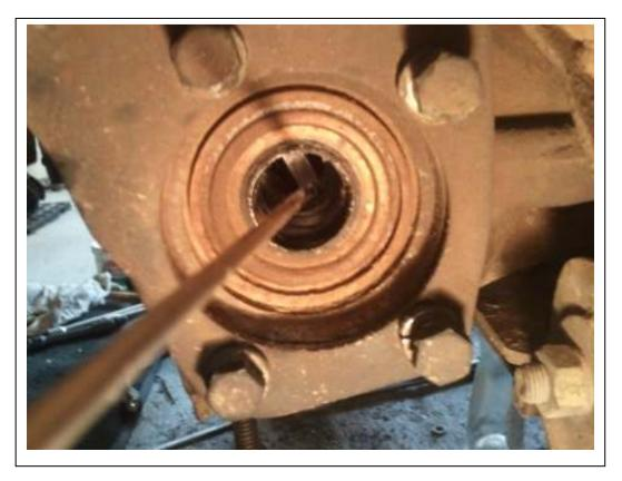
Use a long thin screw driver to line up the splines from outside the diff
