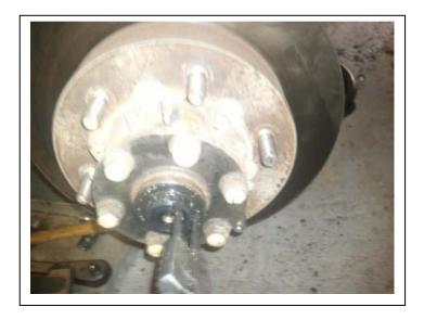
After removing the wheels remove the cap on the front hubs remove the circlip and shim
