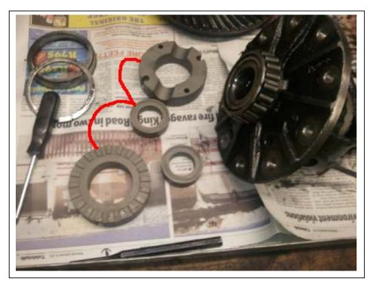
These three components make up one side of the lokker
