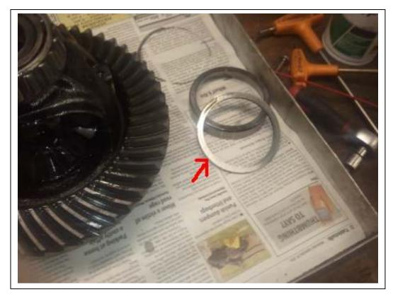
Remember to keep the LHS and RHS bearing races and shims separate
