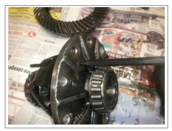
After removing the crown wheel knock out the pin do not remove the pin completely
