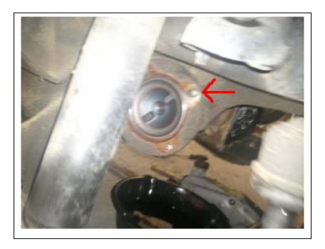
This is the second drive shaft on the RHS I could not remove it by pulling I used a crow bar from the rear side. I also removed the bolts on the bracket to lower the diff
