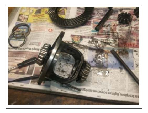
Empty Carrier keep the original shims from the spider gears to use with lokker
