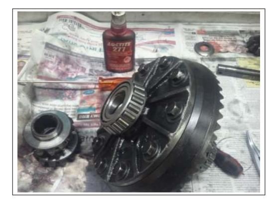
Torque all the bolts to 78-88Nm and apply lock tight
