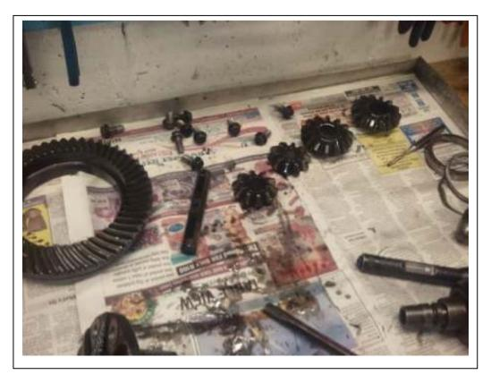
Spider gears removed
