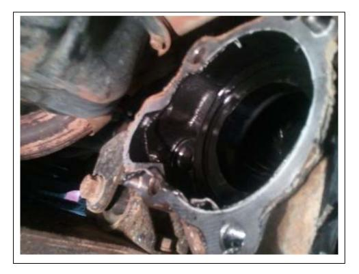
The small shaft fits into this cavity and locates into the diff on the RHS
