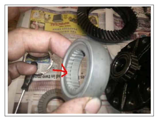
I was a bit confused as to the way this collar went in as the instructions were very vague , once installed you will need to line up the spines with the second part of the lokker in order to slide the drive shaft all the way home
