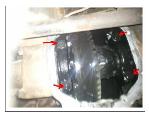
Now after removing the cover on the diff remove the four bolts
