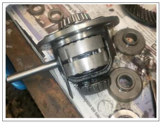
Checking to see if the locker cleared the carrier sometimes one needs to grind a small amount
