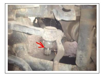
Remove the steering control arm completely
