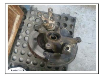
Knuckle removed I separated the ball joint at this point with my air gun and hammer I could not believe how seized on they were.
