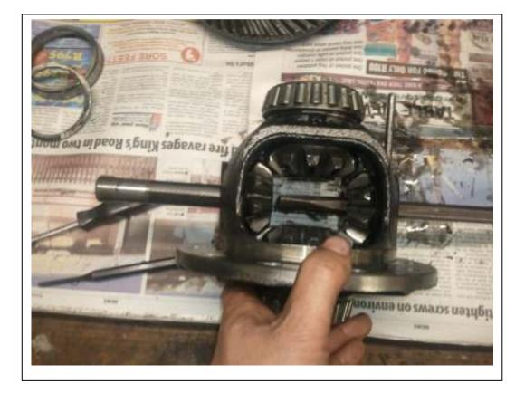
Now you can remove the shaft in order to remove the spider gears
