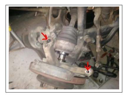
Remove the knuckles on both sides. I could not get the lower ball joints to separate even with my 600Nm air gun on it this was the first time ever that my gun was not able to remove something, I eventually removed the four bolts holding the lower ball joint to the control arm
