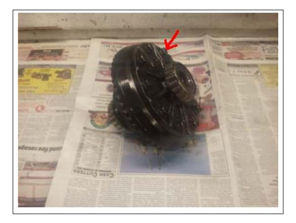
Once the crown wheel is removed you will need to remove all the bolts
