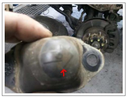
This is the bump stop from the top control arm I removed them as I did this job on my own and was not able to get the bottom and top control arms to connect, with the bump stops removed I could manipulate the two together after loosening the torsion bars this took a huge effort and I battled for ages on this part I never knew I could swear so much, note the arrow on the bump stop it faces towards the engine
