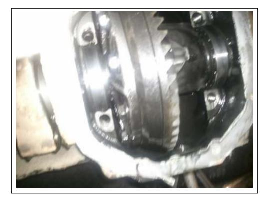
Bolts and bearing retainers removed keep all parts from each side separate so they go back on the correct side. I had to pull and jiggle the crown wheel to release it, be careful not to break the shims on the sides. If you are laying under the vehicle do not let it drop on your head it is rather heavy
