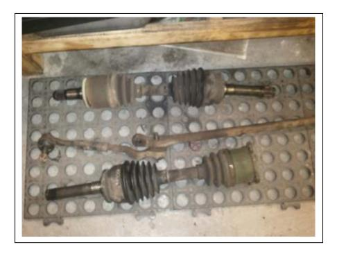
Both outer drive shafts and steering arm removed
