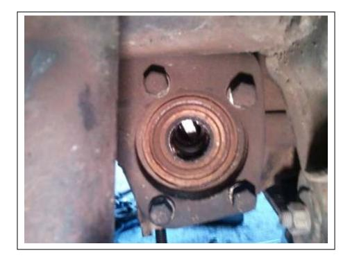
Remove the four bolts on the LHS of the diff in order to pull the diff forward this will give you access to the rear bolts on the front drive clutch
