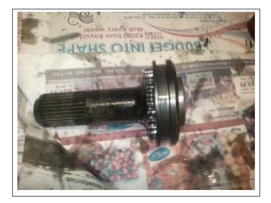
Note the ring gear's narrow side goes towards the shaft
