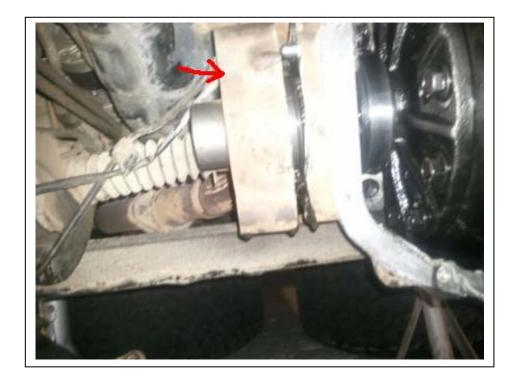
Separating the front drive clutch in order to remove the small third drive shaft on the RHS yes three drive shafts and a clutch???
