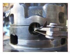
Rotate the Aussie Locker assembly so that the gap between the 2 cam gears can be measured through the cross-shaft holes. Pry the gears apart by installing 2 screwdrivers through cross-shaft holes opposite of each other to ensure gears are seated and maximum gap is achieved. Remove the screwdrivers. Use 2 feeler gauges opposite of each other simultaneously so 'cocking or tilting' of the cam gears is very limited. Average the 2 feeler gauge measurements.
