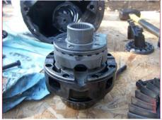
Install one cam gear onto an axle gear already installed non-ring gear half of the carrier. Do not fit the cross shaft.
