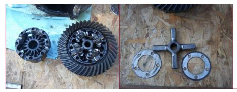
Remove Third member from axle housing, Remove Ring gear bolts and remove ring gear. Remove carrier bolts and split carrier in half.
