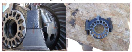
Mark the Bearing Adjusters for installation in same position. Mark the carrier bearing caps for later removal and replacement to the exact same location. Remove the carrier bearing cap bolts, (do not remove the bearing adjuster bolt/retaining clip) remove each bearing cap and bearing adjuster together (may need to tap with hammer in upward motion) keep assemblies separate (ie; left to right for reassembly in same location)
