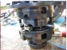
Reassemble the carrier as before with the cross shaft located between the cam gears. Apply locktite to the carrier bolts Ensure the alignment marks on the carrier match. Ensure the pins and springs are aligned before final tightening of the assembly bolts tighten and torque the bolts to 50 ft lb in a cross pattern. Refit and torque the Ring Gear to the carrier.
