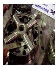
Clean and inspect the thrust washers install the thrust washers on the axle gears. Install the axle gears 1 each into each carrier half ensure the gear spins freely. Install the spacer ring over the center of each axle gear. Install the cross-shaft into one of the carrier half's. With a feeler gauge measure the gap between the cross shaft center block and the top of the spacer ring. This gap should be between 0.006 and 0.020"
