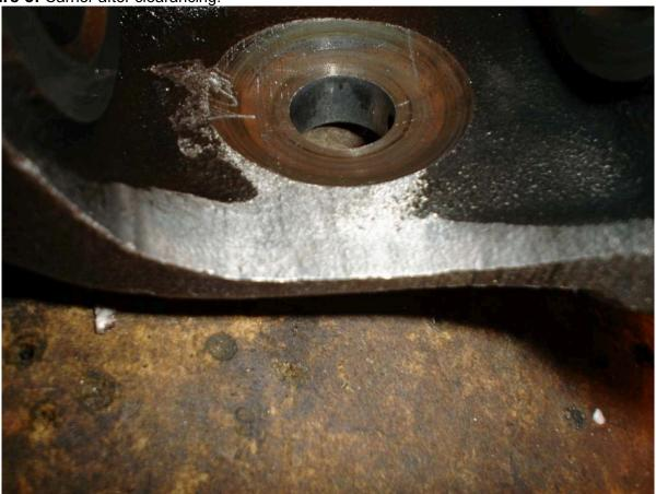
Figure 4: Checking the cross-shaft (pinion shaft) to spacer clearance (.005 - .020).
