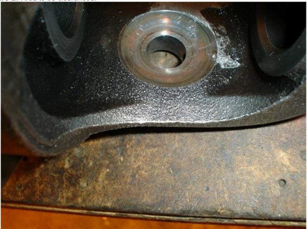
Figure 3: Carrier after clearancing.
