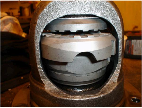
Figure 6: Measuring the center gap (.140 - .170).
