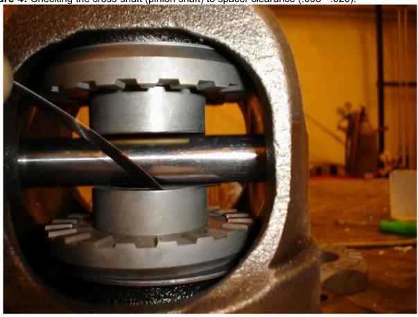
Figure 5: Sliding the 2<sup>nd</sup> cam gear in after clearancing the carrier.
