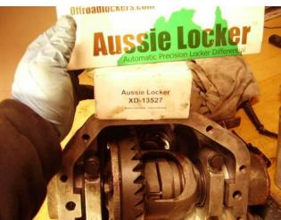
I then reinstalled the carrier into the housing and torque to manufactures specs.
