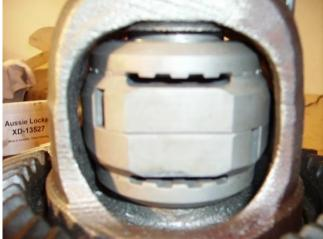
Install the shims from the side gears under the axle gears. Install one set of the axle gears, spacers and cam gears onto the side of the case with the ring gear. Next install the axle gear on the open side of the carrier, then the spacer and cam gear (mine fit without any grinding on the carrier at all but some may require a little clearancing of the window.
