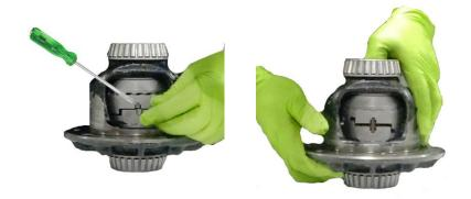
**NOTE:** The springs are firm. Place the spring in the bottom of the pocket, then use a small flat head screwdriver to compress the spring and pop it into the top pocket.
