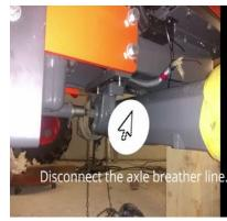
**3.)** Prep vehicle for TORQ Locker install: Disconnect both hydraulic connections from the steering actuator. Disconnect the axle breather line.
