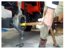
**5.)** Prep vehicle for TORQ Locker install: Remove the pinion gear. Be mindful of the shims inside the axle housing at the differential. Push the differential out of the axle housing from one side.
