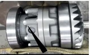
10.) Measure the Center Gap: Torque 2 of the differential case bolts to ensure both halves of the differential are fully seated. Measure the center gap, the space between the two cam gears. The center gap should be between 3,69 mm and 4,318 mm or 0.145" and 0.170". Contact us immediately if your center gap is out of tolerance at <a href="mailto:info@torqmasters.com">info@torqmasters.com</a> Next, torque the differential case bolts to 30-34 NM or 22-24 Ft Lbs.
