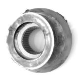
8.) <u>Prep TORQ Locker for Install:</u> Apply medium grease, in a <u>very thin</u> coating, to the teeth of the gears and to the backs of the axle gears. Place the OEM thrust washers on the back side of the TORQ Locker axle gears.
