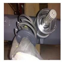
**4.)** Prep vehicle for TORQ Locker install: Remove the Pinion Support. Remove the Pinion seal, snap rings and spacer.
