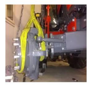
Drain the oil from the axle assembly. Unbolt the steering arm and knuckle assembly, use a motor hoist to move the knuckle out of the work area.
