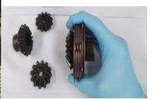
**7.)** <u>Disassemble the Differential:</u> Unbolt and split the differential in half. You will need to punch out the roll pin as far as possible, then cut the roll pin to fully remove it. Save the 2 Thrust Washers from the back side of the drive spider gears for reuse. Remove the spider gears and clutches.
