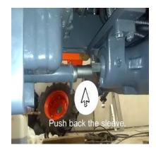
**2.)** Prep vehicle for TORQ Locker install: Remove the 2 front axle shafts. Unbolt and slide the driveshaft sleeve out of the work area. Disengage the driveshaft from the pinion.
