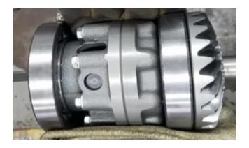
**6.)** Prep vehicle for TORQ Locker install: Remove the differential from the axle housing and place it on a bench.
