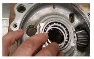
**d.** <u>Lift out the carrier:</u> Lift carrier straight up out of case- there is a shim under it too. The shims must be re-used! Failure to install on reassembly will cause severe damage quickly!
