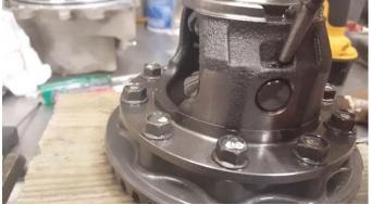
m. <u>Pin driven in:</u> Now peen the pin bore with a center punch to retain pin, and then insert the TORQ Locker springs. Put one end of spring in lower pocket, and push in with fingers. A small screwdriver is helpful to make sure springs are seated in pockets.
