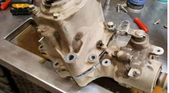
c. <u>Lift off the case halve:</u> Lift the case halve strait up- there's a thrust washer that may be stuck to bearing in case, or on the carrier- locate, and don't lose it. Set case out of way.
