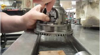
**n.** <u>Installing the Spring:</u> Set the spring in the bottom of the pocket and use a small screwdriver to depress the spring, and your finger to pop the spring into the pocket.
