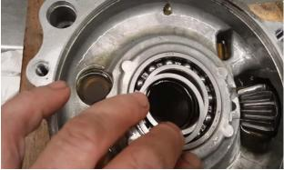
o. TORQ-LOCKER is installed. Set carrier in case, don't forget the thrust differential case shims! (small diameter)
