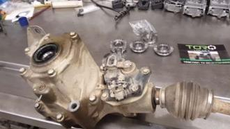
**b.** Remove the case bolts and remove case halve: use the 'pry points' and/or a very thin sharp scraper at the seam to get it to start separating- BE CAREFUL! don't damage the machined surfaces, or drive it in and damage the o-ring seal.
