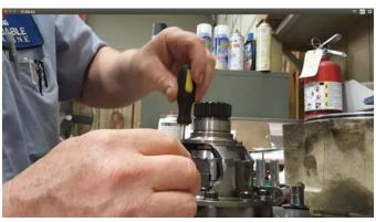
I. <u>Install cross pin:</u> Turn locker to orient cross pin hole and install cross pin with it's retaining pin hole vertical, to line up with the retaining pin hole in carrier. Lift the upper half of TORQ locker to ease cross pin insertion. Align the cross pin retaining pin hole, then drive in retaining pin until about 1/8" below top of bore
