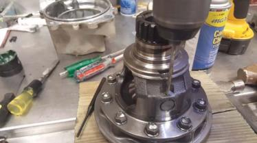
e. Remove the cross pin retaining pin: Locate the retaining pin, and drive it IN gently till it bottoms in bore. Use a 5/32 drill bit to remove peening at top of pin bore- a light touch is all it takes! Don't make the bore bigger. Turn carrier over, and drive retaining pin out.
