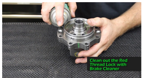
6.) Clean the ring gear bolt holes in the differential case with brake cleaner.
