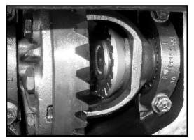
5.) Install Axle 2 Gears: with Thrust Washers on the backs of the axle gears, driver and passenger side
