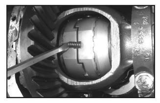
**NOTE:** The springs are Heavy Duty. Try using a flat screwdriver to pry the springs into the pockets. An alternative method is to compress the spring with pliers and insert it about half way into both cam gears, release the pliers, and then tap it into place with a screwdriver handle.
