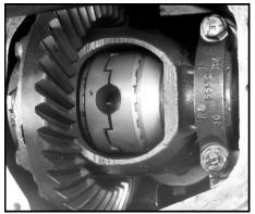
6.) Install First Cam and Second Gear: on Ring Gear side of the case, push it into the grease on the teeth to hold it in position. Notice that next to one of the curved recesses there are pockets that must be facing outward. Install second Cam Gear positioning it so that its projections will slip into the opposing pockets. Slide it in past the left connector until they are flush with each other. Push the right cam gear into the grease to hold it in position
